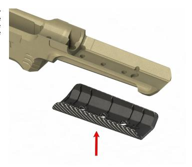
7. Screw the included #8 Phillips head screws into the foregrip by starting with the back hole and the the front hole. Hand tighten both. Once the foregrip is flush torque both down to 10in/lbs.
