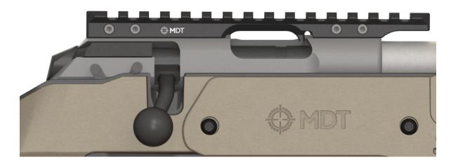
**4.** Torque all screws to 15-20 in-lb. After taking out your CZ for some fun (100-150 rounds), check all four screws and re-torque if necessary.
