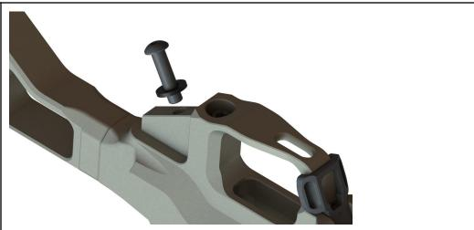
2. Take the pistol grip mount and attach it to the chassis using the pistol grip mounting screw.
