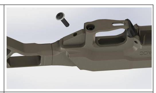
2. Take the grip post and attach it to the chassis using the grip attachment screw and washer.
