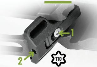
Loosen the front screw (1) with a T10. Insert a magazine and adjust the latch tip height with the bottom screw (2), when the magazine can latch and has a little bit of up/down movement, remove the magazine and tighten the front screw.
