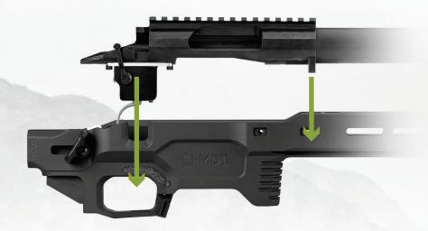
Apply rearward pressure on the chassis with the barrelled action. While maintaining pressure, tighten the barrelled action in place with the action screws. Then, starting with the front screw, torque both screws to 65 in-lbs.
